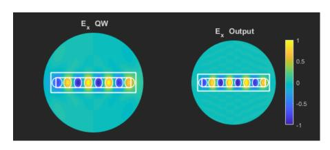
Patterning of relief arrays at the outcoupling facet to ensure single mode emission!
