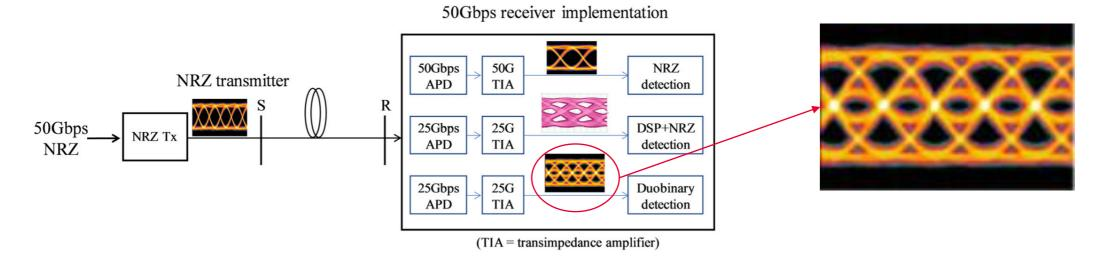
• Received binary signal becomes almost a three-level signal, similar to an **electrical Duobinary sequence**
