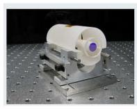
Stabilization of laser frequency on high-finesse Fabry-Pérot cavities and **hertz-wide lasers**, needed for high-resolution spectroscopy.
